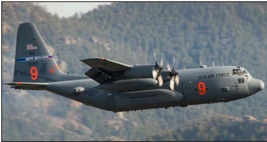
A C-130 from the 152nd Airlift Wing equipped with U.S. Forest Service MAFFS II (Modular Airborne Fire Fighting System) positions to drop water as part of a MAFFS training and recertification at Grand Canyon Hills, Colorado, May 6, 2019. Air National Guard and Air Force Reserve airmen from Wyoming, Colorado, California and Nevada train together annually with the U.S. Forest Service for aerial firefighting.
